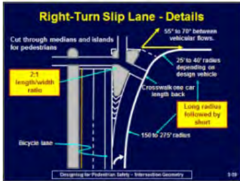
Recommended design for right-turn slip lane.
