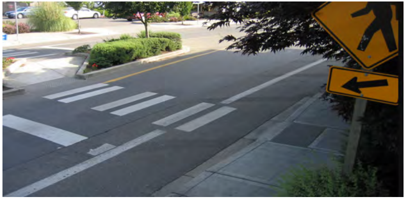
The enhancements shown in this rendering of a midblock crosswalk include high-visibility markings, curb extensions, in-street pedestrian crossing signs, lighting, and warning signs. Federal Highway Administration.
