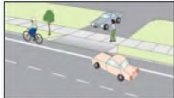
Driveways built like driveways encourage low-speed turns and encourage motorists to yield to pedestrians.
