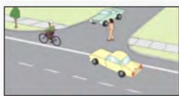
Driveways built like intersections encourage high-speed turns.
