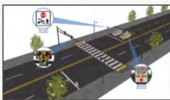
Pedestrian Hybrid Beacon installation shown with accompanying signs and pavement markings. Federal Highway Administration.
